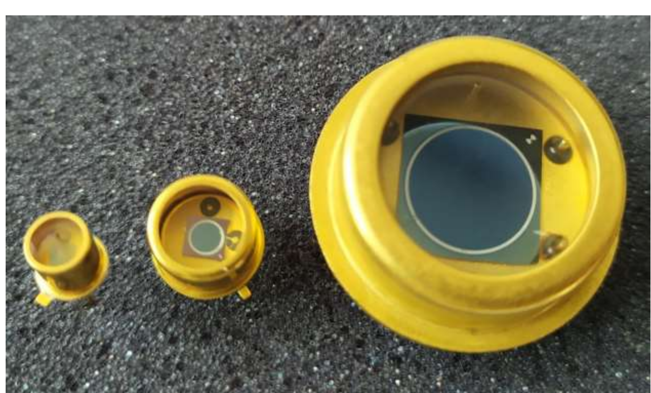
Three different active area surfaces of the PIN diodes.
